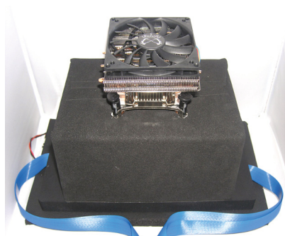
Figure 4: A box with two Peltier cooling elements provides protection against ambient light and allows stable and reproducible temperature conditions.
